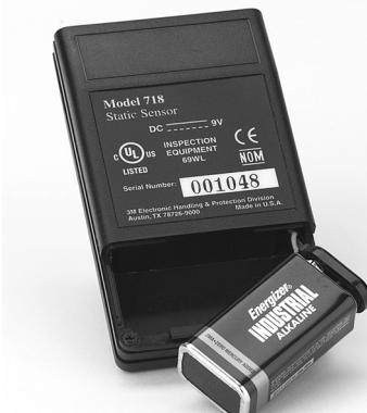
2.2.3 Connect the two, and place the connected battery into the housing by inserting the connector end first, then following up with the other end of the battery.
